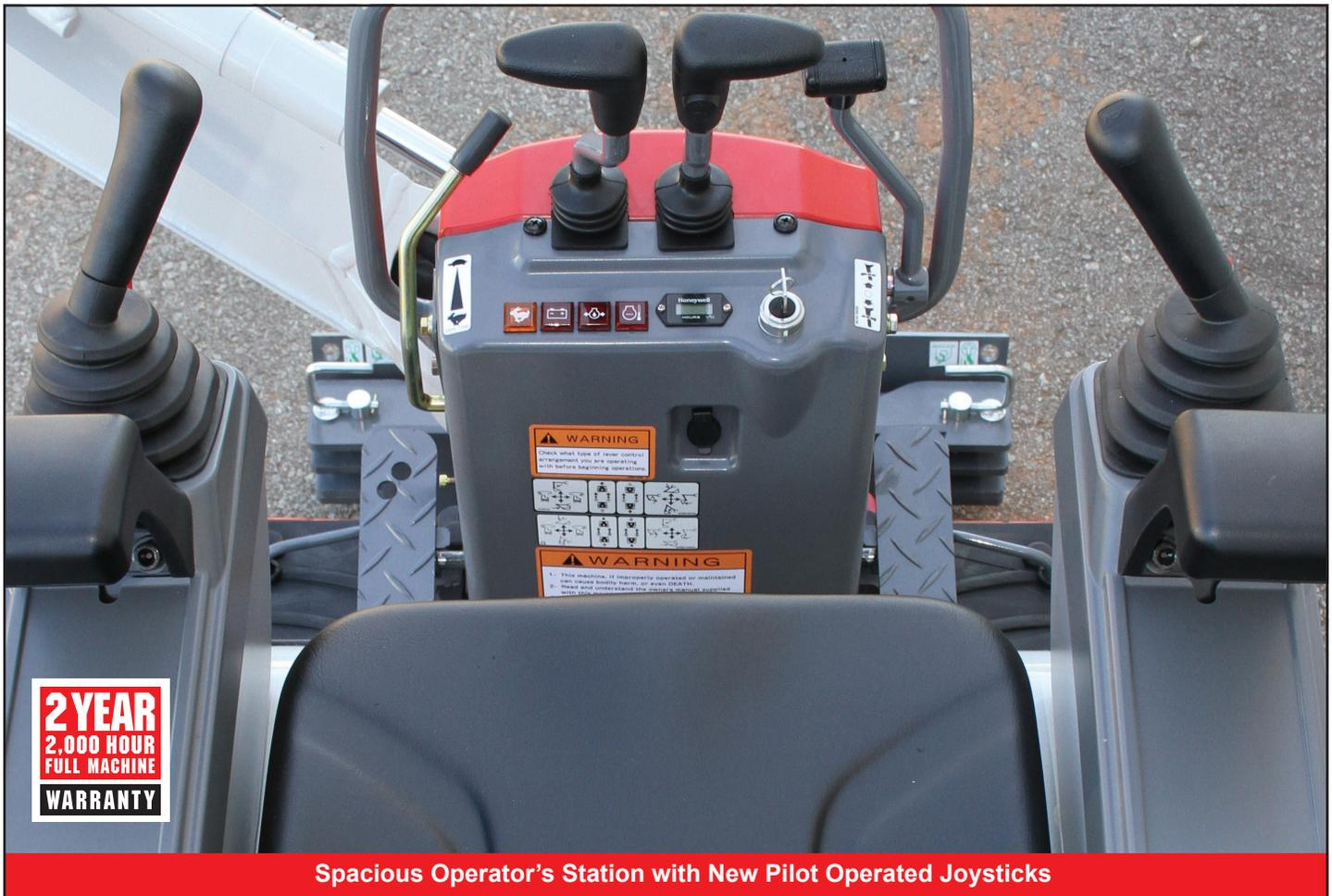
**Spacious Operator's Station with New Pilot Operated Joysticks**
